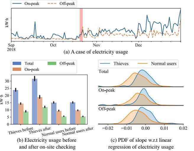
**Figure 2: A study of micro-level factors and electricity theft.** (a) presents a case of electricity usage with the red bar indicating the time at which the thief was caught. (b) presents the statistics of all users pertaining to electricity usage before and after on-site checking, while the trends of the usage are shown in (c). We can therefore see that the behaviors of electricity thieves are different from those of normal users.
