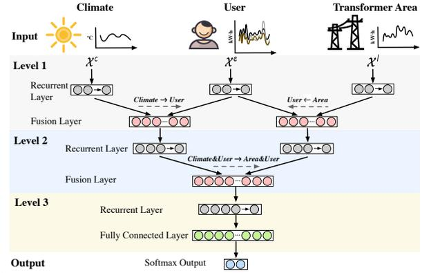
**Figure 6: Architecture of HEBR.** Given a multi-source observation sequence (climate, area and user), HEBR constructs a three-level framework: at each level, different sequences are inputted into different recurrent layers respectively, the latent representations of which are fused in pairs. Dashed lines indicate the direction of the fusion. The last layer outputs the probability of electricity theft.
