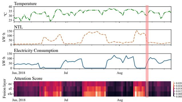
**Figure 8: A case study of the attention operator shown together with different fusion layers ( $\alpha^{ec, el, elc}$ ). The upper rows present different multi-source observation sequences, while the red bar indicates the time at which the electricity theft was detected. The lower row presents the score vector of the attention operator by heat map.**
