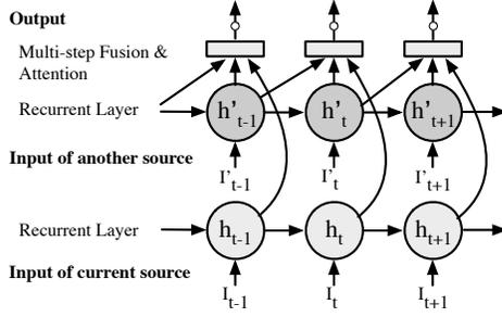
**Figure 7: The architecture of recurrent and fusion layers on multi-source sequences. The sequential inputs of another source  $I'$  are integrated into the current ones  $I$  by means of the above architecture, which is a uniform component in Figure 6.**
